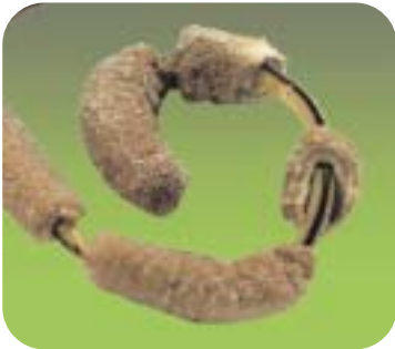
Encrustation: Formation of a mineralized phosphate salt deposit on ureteral stents after an indwelling time of only a few weeks. These deposits cause complications.
